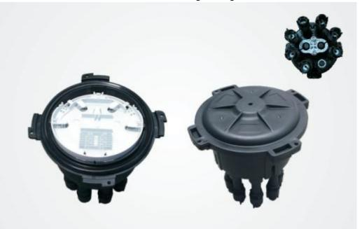
**FOSC400A12** fiber optic splice closures are specially designed to protect joints of optic cable. Excessive fibers can be stored in storage baskets behind the splice trays. The optical fibers are fusion on sides of the tray. One tray can splice 12 fibers; Available for 1 trays to splice total 12 fibers. Adopt modified PP material, with anti-UV, anti-aging and corrosion resistance material. Good quality and long service life. It is reusable.
